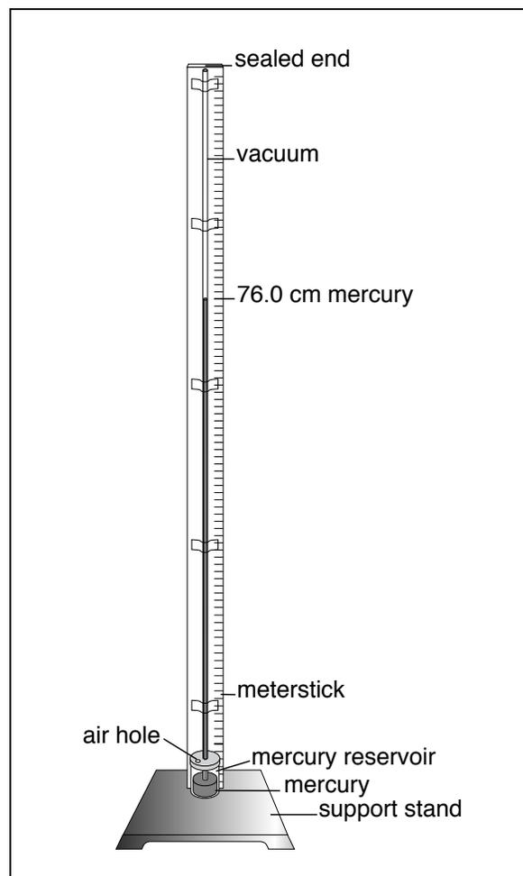
Figure 1. A mercury barometer
