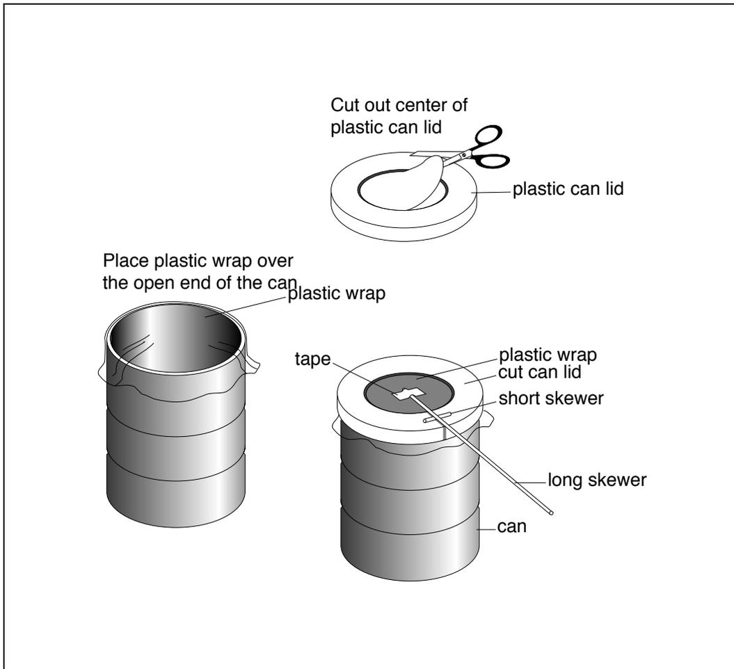
Figure 2. A tin-can barometer
